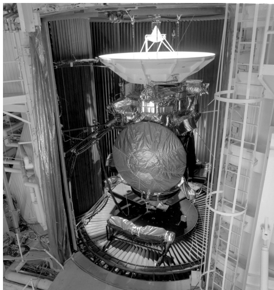
Cassini-Huygens in the test chamber at the Jet Propulsion Laboratory.
